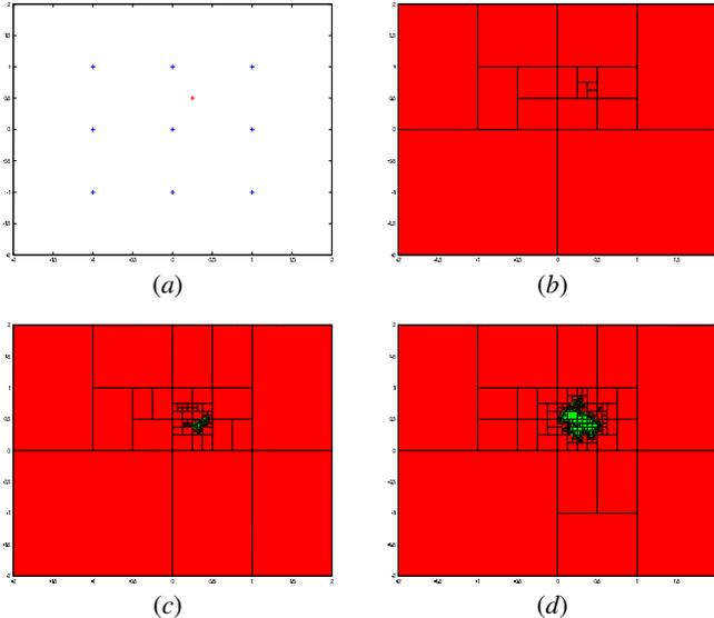
**Fig. 2.** Considered network of 9 sensors (blue) and one source (red) (a); Solution obtained using a centralized estimation technique for  $q = 0$  (b),  $q = 1$  (c), and  $q = 2$  (d); all plots are in  $[-2, 2]^2$
